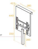
0.8-mm thick folded sheet steel cable riser
